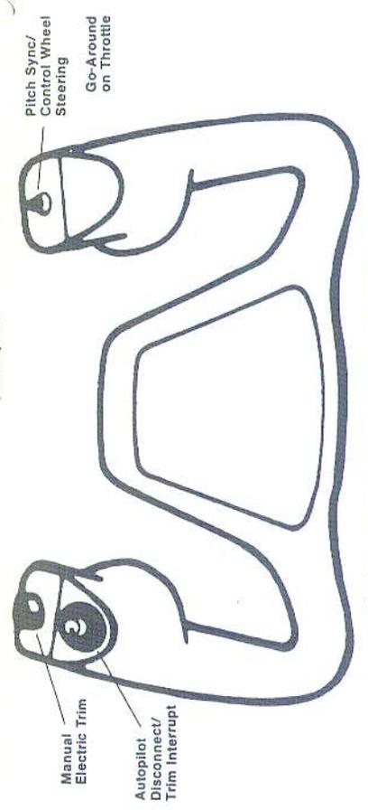
Typical Control Wheel Switch Arrangements
